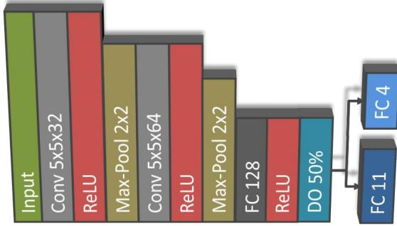
Figure 3: **Cropped LineMOD Task Network:** Simple LeNet-like architecture followed by a dropout layer with a 50% rate and outputting both a class and pose vector.
