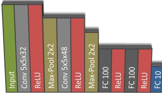
Figure 1: **MNIST Classifier:** Simple LeNet-like architecture, where 2 convolutional layers followed by ReLUs and max-poolings are finalized by 3 fully-connected layers.
