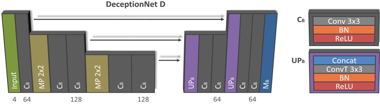
Figure 4: **DeceptionNet architecture.** Our network features a typical encoder-decoder architecture. The encoder part consists of 2 consecutive downsamplings followed by a sequence of convolutional blocks  $C_B$ . The decoder part shares a similar architecture for all presented augmentation modules. Arrows show the skip connections between blocks.
