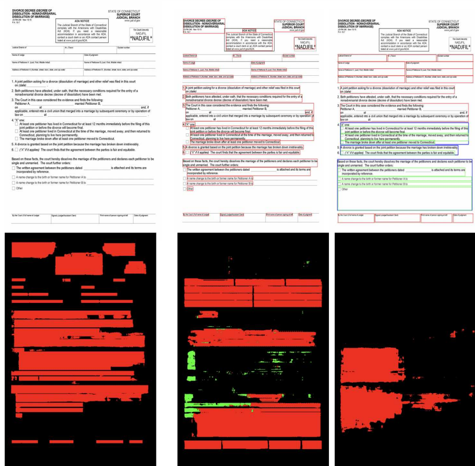
Figure 4. Visualization : Top row shows sample form image (left), bounding box of textblocks (middle - red), text fields (right - red), choice fields (right - green) and choice groups (right - blue) predicted by our method. Bottom row shows MFCN segmentation masks - textblocks (left), text fields (middle - red), choice fields (middle - green) and choice groups (right).
