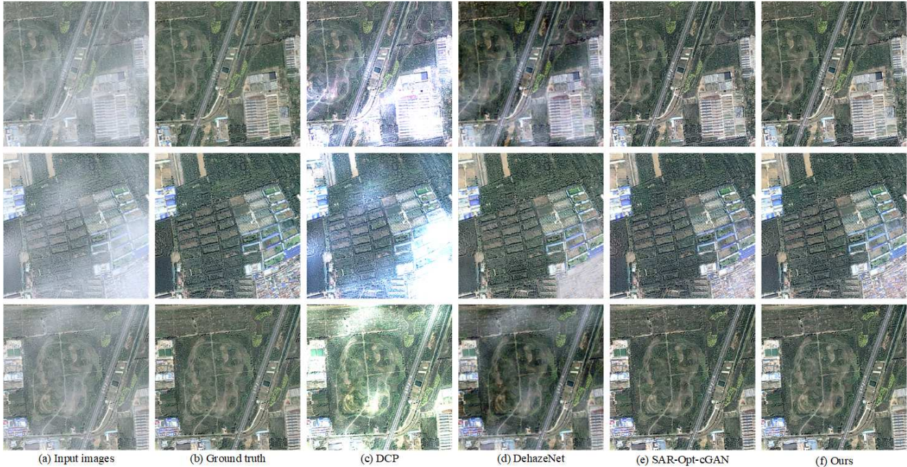
Figure 4. The visual effects of different methods implemented in our dataset. From left to right: (a)Input images, (b)Ground truth, (c)DCP, (d)DehazeNet, (e)SAR-Opt-cGAN, (f)Ours. The generative methods e.g. SAR-Opt-cGAN and ours generate more clear haze-free images than the methods based on atmospheric scattering model e.g. DCP and DehazeNet. Our method conditions the GAN model on additional SAR information and performs better than [13] whose name is called SAR-Opt-cGAN but actually use the normal GAN).
