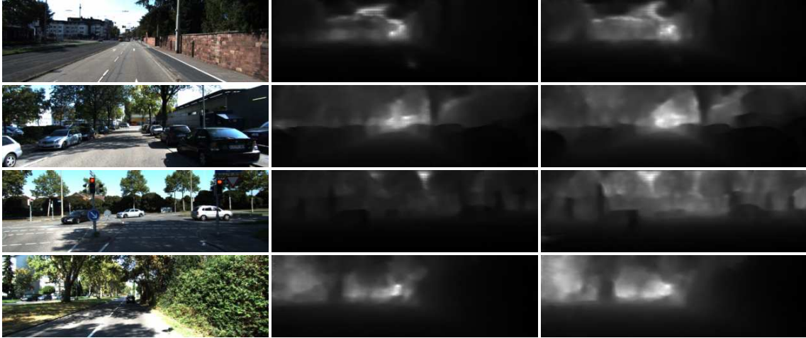
Figure 6: Qualitative examples of depth estimation for one step (middle) and two steps (right) depth estimation through depth estimation network. Note that the only difference between them is the compositional re-estimation.
