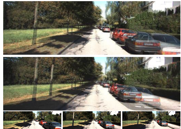
Figure 1: An illustration of the problem of large displacement between two views in pose estimation with the view synthesis formulation. The 3rd row shows three consecutive frames in a video. The 1st row shows the difference between the left and middle frames. The 2nd row shows the difference between the middle and right frames. When the displacement of two views is large, the assumption made by the view synthesis no longer holds. In this paper, we propose an alternative approach that splits the estimation into smaller pieces and re-estimate the transformation through a compositional transformation estimation.
