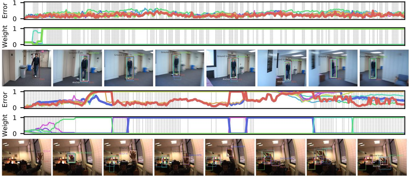
Figure 6. **Tracking examples.** The top is “BlurBody” in OTB2015 and the bottom is “Hand” in Tcolor2018. For the picked-up frame, we annotate ground truth (black), the proposed method (red), and only for anchor frames, we annotate the detected bounding box (white). The expert which has the highest weight is also annotated. In the error and weight graph, gray vertical lines show anchor frames.
