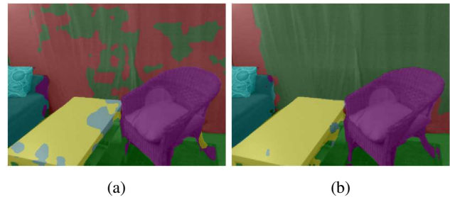
Figure 1: (a) Even the state-of-the-art method DeepLabV3+ trained with training data from SUNRGB-D makes many mistakes when segmenting an image outside the SUNRGB-D dataset. (b) After exploiting geometric constraints on an unlabeled sequence of the new scene, our semi-supervised S4-Net approach predicts much better segmentations.
