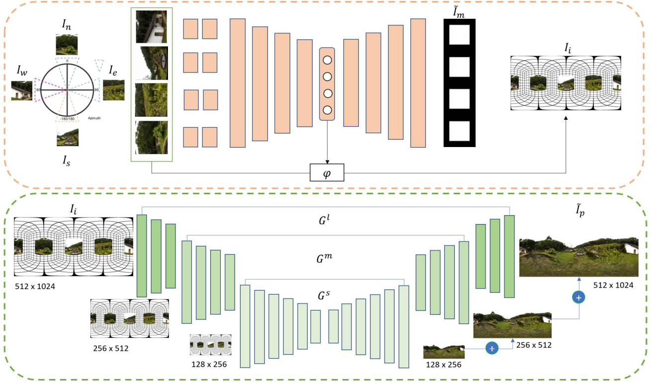
Figure 2: The architecture of the proposed network. We show the visualization of the relative FOV estimation network (top) and panorama synthesis network (bottom). The network takes sequence of 4 input images to estimate the equirectangular panorama with missing pixels. This equirectangular panorama is then used as the input for the panorama synthesis network. The synthesis process is done on each scale on small, medium, and large.
