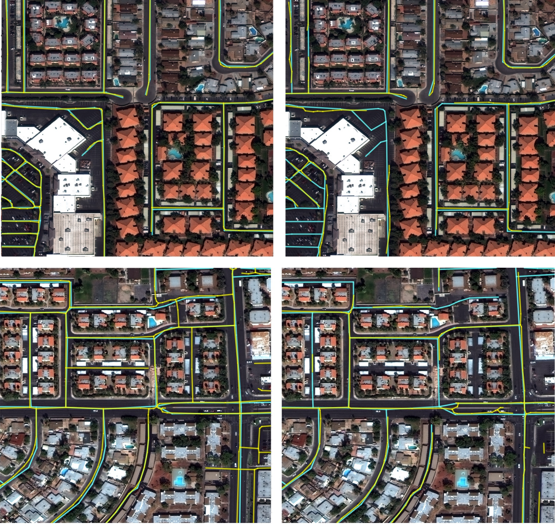
Figure 2: SpaceNet compared to OSM. Road predictions (yellow) and ground truth SpaceNet labels (blue) for a sample image chips, with SpaceNet models on the left and OSM-trained models on the right. Top: SpaceNet model predictions (left) score \text{APLS}_{\text{length}} = 0.60 , while OSM model predictions (right) yield \text{APLS}_{\text{length}} = 0.48 . Bottom: SpaceNet model predictions (left) score \text{APLS}_{\text{length}} = 0.92 , while OSM model predictions (right) yield \text{APLS}_{\text{length}} = 0.37 .
