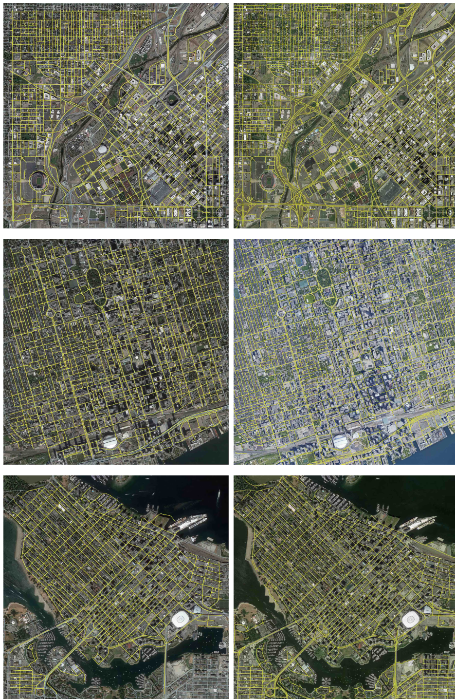
Figure 4: RoadTracer / CRESIv2 . Performance comparison between RoadTracer (left column, OSM labels in gray, predictions in yellow [2]) and CRESIv2 (right column, predictions in yellow) for various cities. From top: Denver, Toronto, Vancouver.
