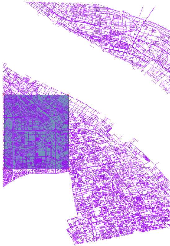
Figure 1: SpaceNet road vector labels over Shanghai (purple). The label boundary is discontinuous and irregularly shaped, so we define rectangular regions for testing purposes (e.g. the blue region denotes test region Shanghai_0).
