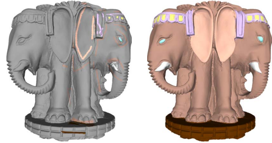
Figure 9. Colorizing a large noisy object. Since the pattern instances are not identical, the user marks on a few instances of the same pattern and the learning is based on all these scribbles.
