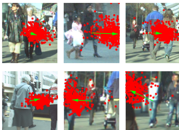
Figure 1: We estimate the velocity of the pedestrian in image coordinates by learning a mapping from image features to pedestrian velocity using a Hough Random Forest (RF) framework. The green arrow indicates the ground truth velocity of the pedestrian, and in red we plot the votes made by the corresponding leaves of the learned RF.
