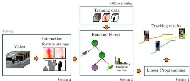
Figure 2: Diagram of the proposed approach. From a new video, we compute interaction feature strings (Section 2) and use them to train a Random Forest (Section 3), which will output the estimated pedestrian velocity. This information is used directly for tracking in a Linear Programming framework (Section 4).
