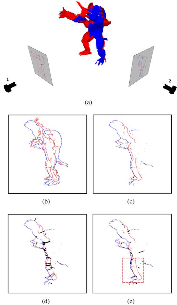
Figure 3. (a) Front range scan (red) and side range scan (blue) of the Stanford Armadillo. (b)  $\mathcal{C}_{1 \rightarrow 2}$  (red) and  $\mathcal{C}_2$  (blue). (c)  $\mathcal{C}_{1 \rightarrow 2}^p$  (red) and  $\mathcal{C}_{2/1}^p$  (blue). (d) Bijective correspondences (black line) found in 3D. (e) Bijective correspondences (black line) found in 2D with red rectangle indicating mismatches
