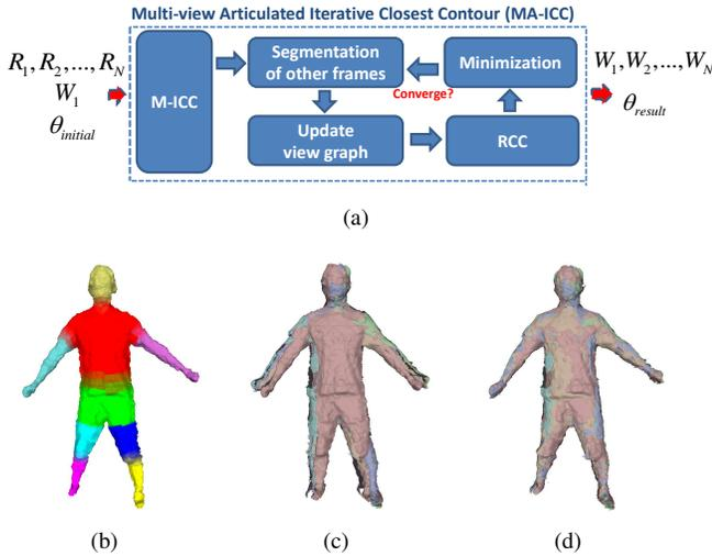
Figure 5. (a) Our MA-ICC method. (b) Segmentation of human body into rigid parts. (c) Registration result after our M-ICC method. (d) Registration result after our MA-ICC method.
