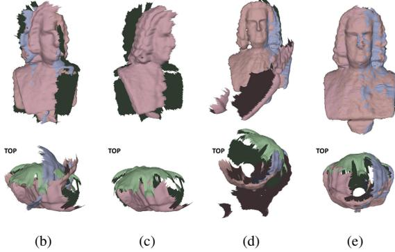
Figure 4. (a) Our M-ICC method. (b) 4 range scans of a Bach head statue taken approximately at  $90^\circ$  apart, with limited overlap and poor initialization. (c) Initial right range scan and back range scan barely overlap and have a large rotation error. (d) Result of pairwise registration using standard ICP algorithm. (e) Result of our M-ICC method.
