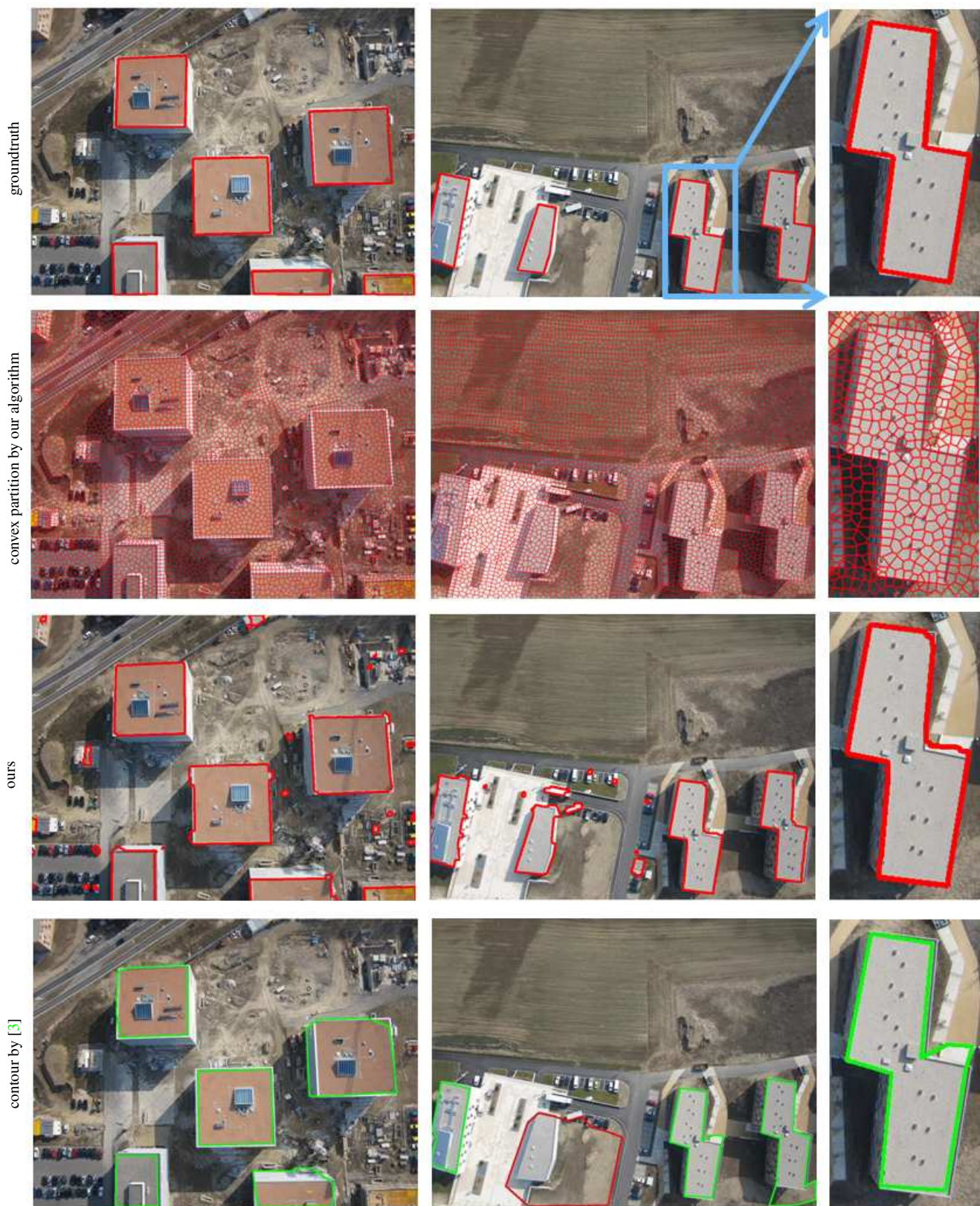
Figure 2. Object polygonization. Visual comparison of polygonal contour extraction by our method and by [3] from aerial images. The class of interest corresponds to building roofs.
