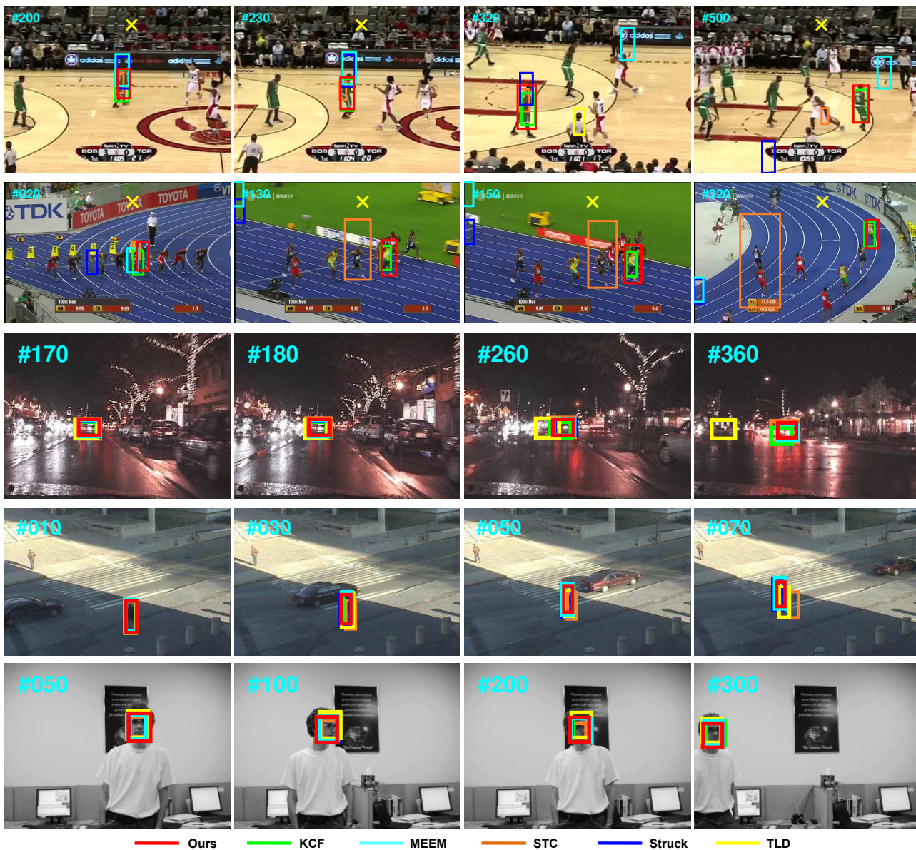
Figure 2. Tracking results of our proposed algorithm, KCF, STC, and TLD methods on six challenging sequences (from top to down are Basketball , Bolt , CarDark , Crossing , and David2 , respectively). A case of tracking failure is denoted by \times .
