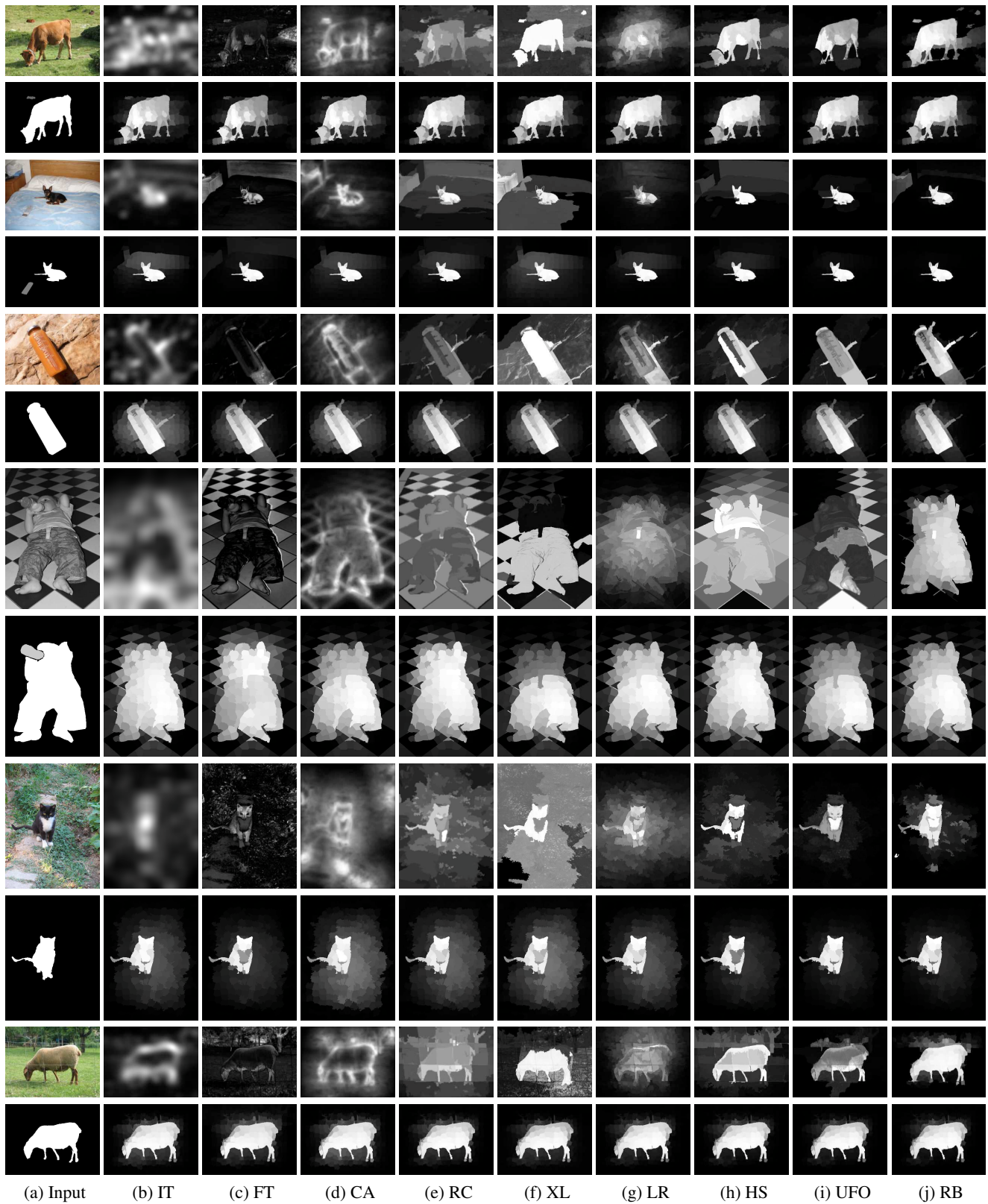
Figure 10. Comparison of different saliency maps generated by nine state-of-the-art methods and optimized by Single-layer Cellular Automata on PASCAL-S. The saliency maps in the odd rows are original results. The saliency maps displayed in the even rows are the optimized results. Input images and ground truth are presented in the first column.
