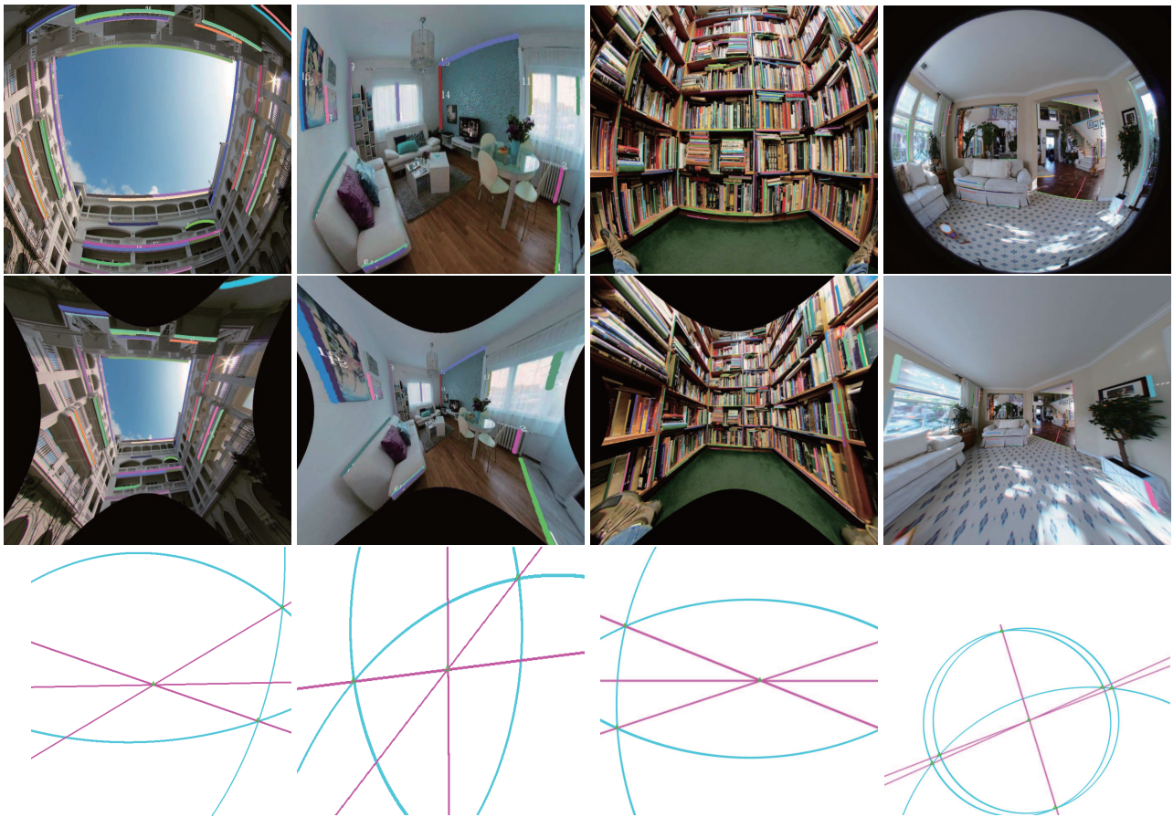
Figure 2. Circular arcs selection results: The first row is the clustered circular arcs for source image. The second row is the corresponding line information in undistorted perspective image plane. And the last row depicts the selected circular arcs for intrinsic parameters estimation.
