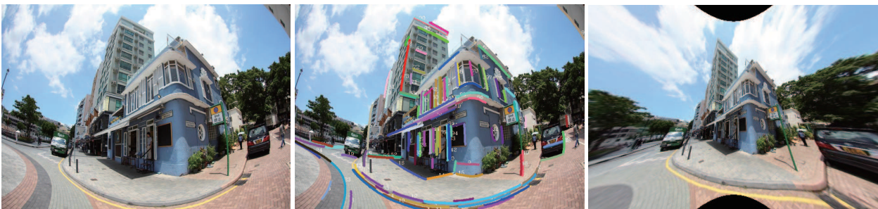
Figure 9. Failed Example # 2: Wrongly rectified result due to the circular structure of target object. The yellow line itself is the circular arc in real scene and this makes the incorrect rectified result.
