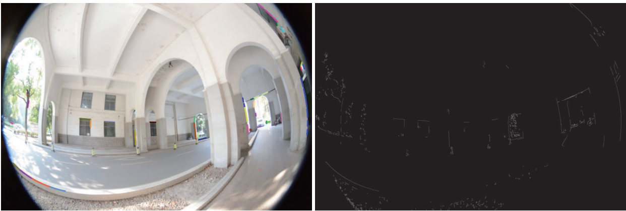
Figure 8. Failed Example # 1: Poorly detected circular arcs due to low texture regions in source image. The Canny edge detector could not perform well as expected, thus leading to fewer clustered circular arcs in source image.
