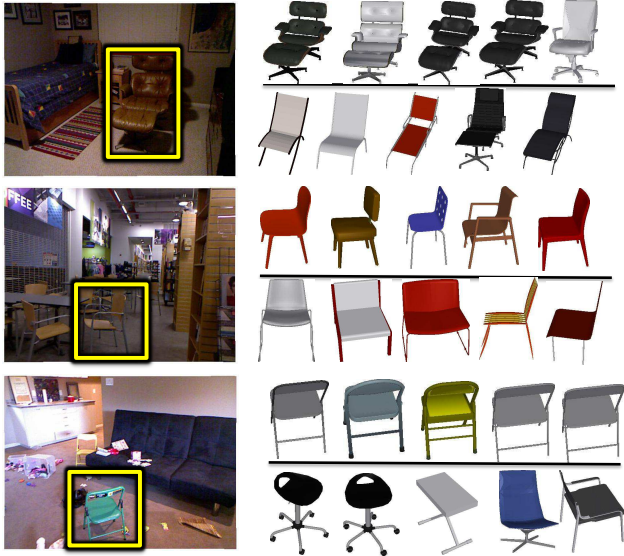
Figure 6. For each example, the top row shows CAD models retrieved using fc-7 of Pose Network and the bottom row shows the result of nearest-neighbor retrieval using predicted surface normals.
