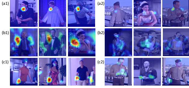
Figure 2. Examples of response maps of different images to the same feature channels. (a) A feature channel for the neck. (b) A feature channel for the left wrist. (c) A feature channel for the left lower arm.
