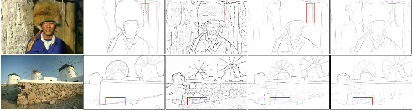
Figure 5. Edge detection examples on BSDS500 [1]. From left to right: input image, ground truth, Sketch Token [27], DeepContour [35], LMLE-kNN. Note the visual differences in the red box.
