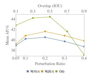
Figure 4. Performances of different max-pooling schemes. The blue and yellow lines are random sampling 10 and 20 samples per box with different perturbation ratios (bottom). The green line shows the performances of different overlap thresholds (top) for adding orginal proposals. Best viewed in color.
