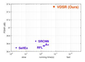
Figure 1: Our VDSR improves PSNR for scale factor  $\times 2$  on dataset Set5 in comparison to the state-of-the-art methods (SR-CNN uses the public slower implementation using CPU). VDSR outperforms SRCNN by a large margin (0.87 dB).
