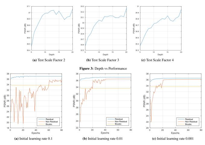
**Figure 4:** Performance curve for residual and non-residual networks. Two networks are tested under 'Set5' dataset with scale factor 2. Residual networks quickly reach state-of-the-art performance within a few epochs, whereas non-residual networks (which models high-resolution image directly) take many epochs to reach maximum performance. Moreover, the final accuracy is higher for residual networks.
