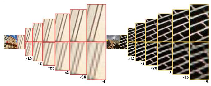
Figure 5: (Top) Our results using a single network for all scale factors. Super-resolved images over all scales are clean and sharp. (Bottom) Results of Dong et al. [5] ( $\times$ 3 model used for all scales). Result images are not visually pleasing. To handle multiple scales, existing methods require multiple networks.
