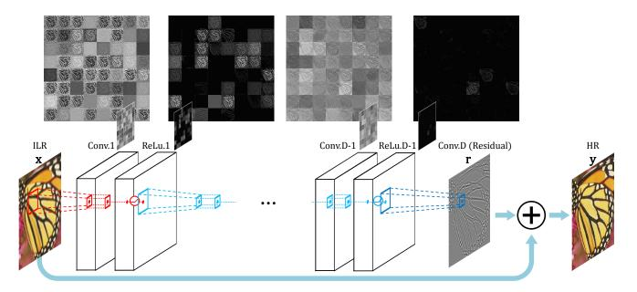
**Figure 2:** Our Network Structure. We cascade a pair of layers (convolutional and nonlinear) repeatedly. An interpolated low-resolution (ILR) image goes through layers and transforms into a high-resolution (HR) image. The network predicts a residual image and the addition of ILR and the residual gives the desired output. We use 64 filters for each convolutional layer and some sample feature maps are drawn for visualization. Most features after applying rectified linear units (ReLu) are zero.
