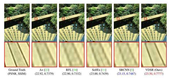
Figure 6: Super-resolution results of "148026" (B100) with scale factor ×3. VDSR recovers sharp lines.
