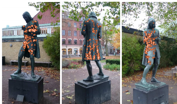
Figure 4. The figure shows three frames of the Linnaeus sequence. Also shown are the tracked Harris points (orange circles) and the reprojected points (white dots) using the proposed method. For visibility a random subset of 250 points are shown
