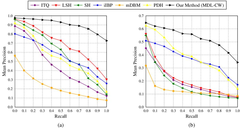
Figure 7. Results of category retrieval for all the query types (a) text-to-image and (b) image-to-image queries on PASCAL-Sentence dataset. Our method using unsupervised fine-tuning is compared with state-of-the-art supervised methods.
