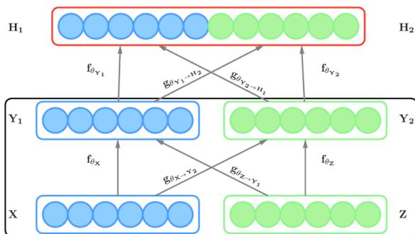
Figure 5. Using last layer representation of the multimodal input as target for unsupervised fine-tuning of Deep Multimodal Network with Cross Weights.
