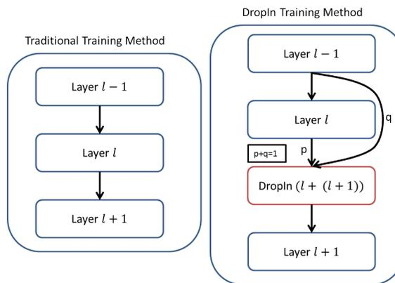
Figure 1: Diagram of traditional vs DropIn training method. The DropIn method sends activations from Layer  $l - 1$  to Layer  $l + 1$  (thus skipping Layer  $l$ ) with a ratio  $q = 1 - p$  and from Layer  $l$  to Layer  $l + 1$  with a ratio  $p$ .
