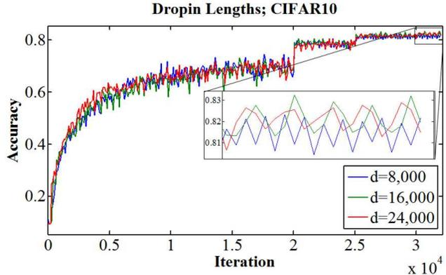
Figure 4: Test data classification accuracy while training the 11-layer CIFAR-10 architecture with DropIn. The curves show classification accuracies for different dropin\_lengths,  $d$ . (Best viewed in color)
