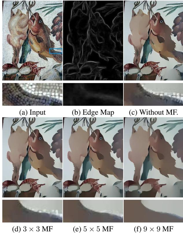
Figure 4. Different median filter size will affect the texture removal result around edges and thus the filter size should be adjusted according to the scene content.
