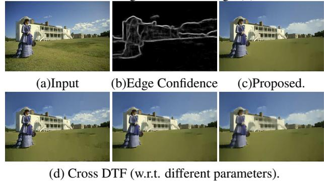
Figure 3. Direct use of the edge confidence as the guidance may introduce visible artifacts or blur the image as shown in (d) (zoom in for details). (c) shows that the combination of the image gradients from (a) and the edge confidence in (b) can effectively suppress the potential artifacts due to imperfect edge detection.
