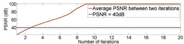
Figure 5. Average PSNR values computed from filtered images between every two iterations. PSNR values larger than 100 was shown as 100 for better visualization (as it can be infinity).
