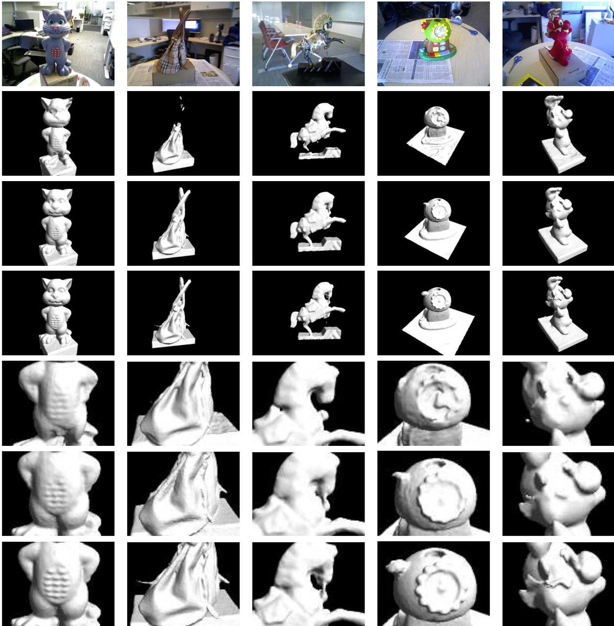
Figure 7. Visual comparison of generated meshes. Row 2-4 are meshes generated by KinFu [19], RGB-D alignment only (i.e. our approach with silhouette consistency term disabled) and joint optimization. Row 5-7 show close-up views of the respective models.
