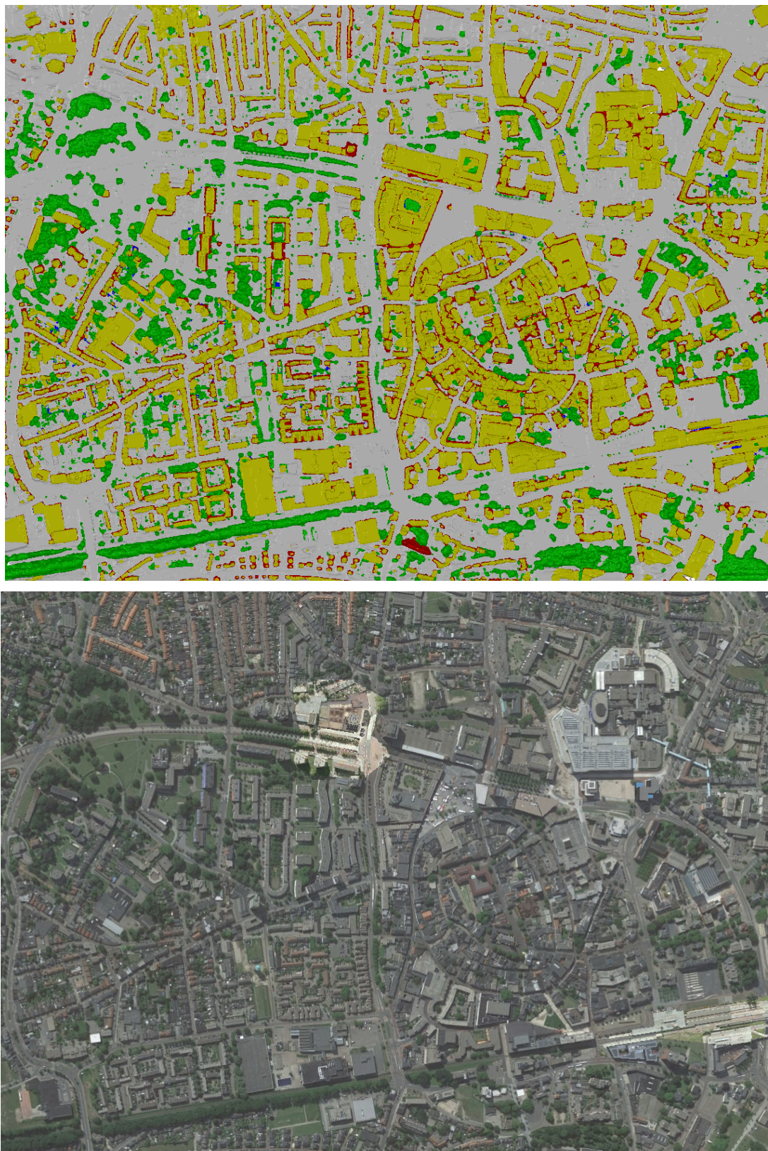
Figure 1. Additional Visualizations. Top : orthographic birds-eye view of the complete Enschede model. Bottom : independent Google Earth image of the same area. Colors indicate ground ( gray ), building ( red ), roof ( yellow ), vegetation ( green ) and clutter ( blue ).
