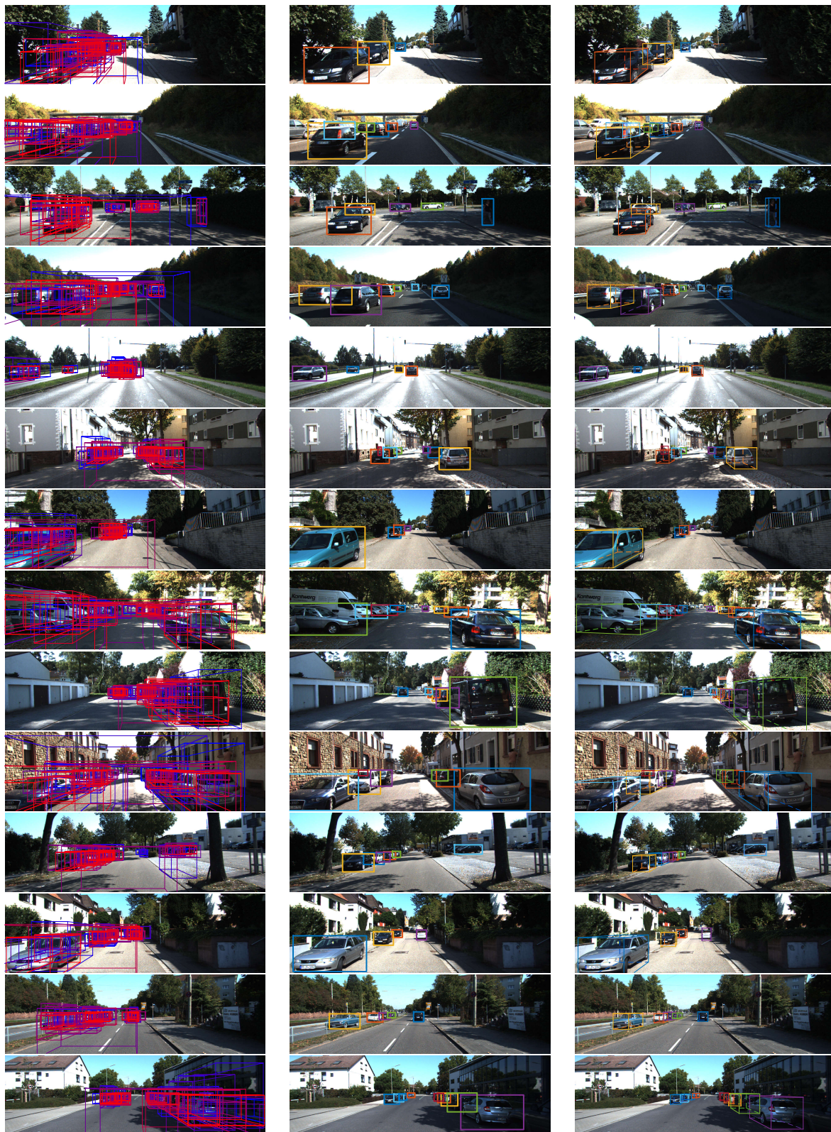
Figure 13: Qualitative examples of detections results for Cars: (left) top 50 scoring proposals (color from blue to red indicates increasing score), (middle) 2D detections, (right) 3D detections.
