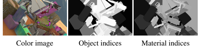
Figure 4. Segmentation data: object indices are unique per scene. Material indices can be shared across objects, but can be combined with the object indices to yield an oversegmentation into parts.
