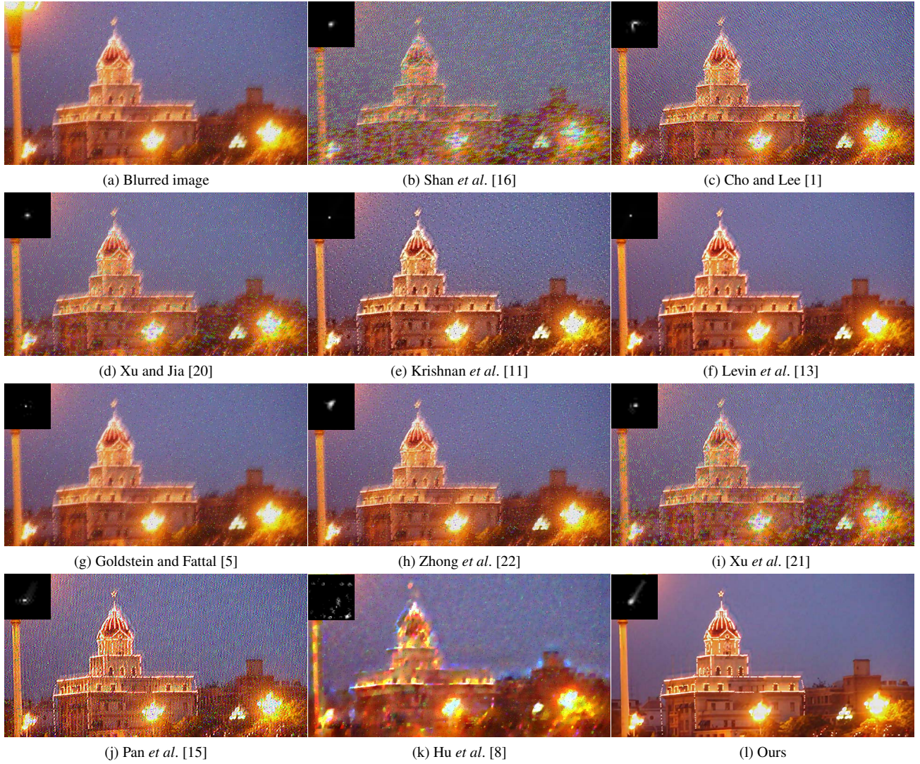
Figure 18. Deblurred results on one blurred image with large saturated areas ( e.g. , light blobs) and noise. State-of-the-art deblurring algorithms [16, 1, 20, 11, 13, 5, 22, 21, 15, 8] fail to generate clear images. In contrast, our method generates a clear image with fine details.
