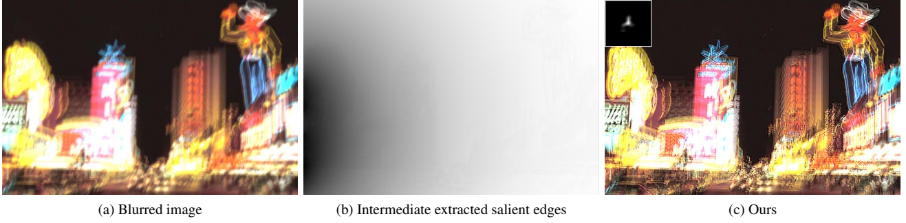
Figure 8. The proposed method is likely to fail when edges are not extracted from intermediate latent images.
