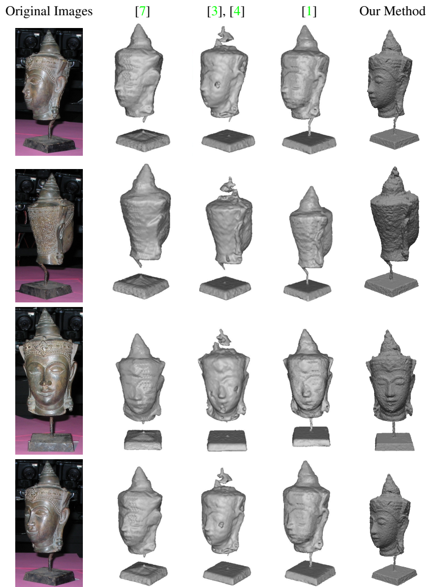
Figure 2: Rendering of the results on the "Head" dataset. The columns from two to four are reported by [1]. It has been shown in [1] that ray information can help in reconstructing the thin pole on which the head is mounted. Our algorithm successfully reconstructs this pole as well.
