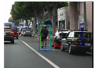
Figure 9: Example annotation errors, a subset of false positives. False positives in red, original annotations in blue, ignore annotations in dashed blue, true positives in green, and ignored detections in dashed green (because they overlap with ignore annotations).
