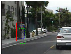
Figure 7: Example localisation errors, a subset of false positives. False positives in red, original annotations in blue, ignore annotations in dashed blue, true positives in green, and ignored detections in dashed green (because they overlap with ignore annotations).
