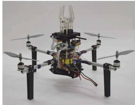
Figure 1. Picture of the aerial robot platform, previously developed in our research group, with a robotic hand on the top of the airframe.
