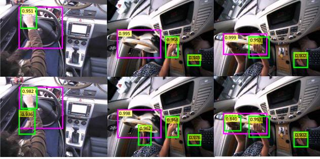
Figure 3. An comparison of our proposed MS-FRCNN against F-RCNN [18] on detecting small objects like hands. The 1<sup>st</sup> row: F-RCNN [18]. The 2<sup>nd</sup> row: our MS-FRCNN
