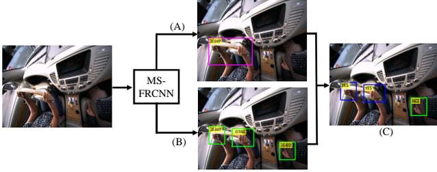
Figure 4. A flowchart of our hand on wheel detection by applying the proposed MS-FRCNN (A): Steering wheel detection, (B): Hand detection, (C): Hand on wheel detection
