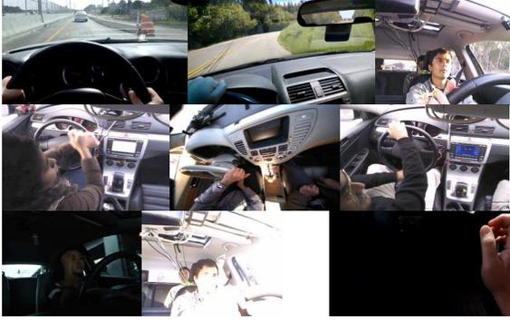
Figure 9. The cases when our hands on wheel detection algorithm fails. 1<sup>st</sup> row: hand occlusion; 2<sup>nd</sup> overlapping; 3<sup>rd</sup> under/over illumination
