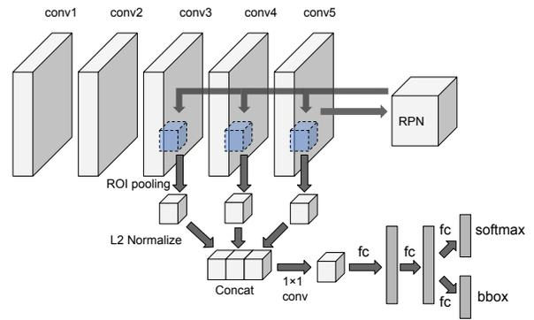
Figure 2. Our proposed Multiple Scale Faster-RCNN (MS-FRCNN) framework.
