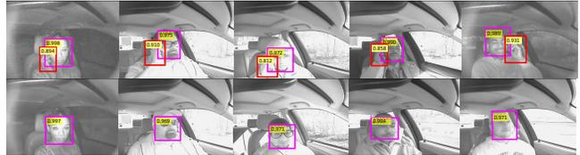
Figure 7. Some examples of our cell-phone usage detection. The 1<sup>st</sup> row: cell-phone is being used. The 2<sup>nd</sup>: there is no cell-phone used
