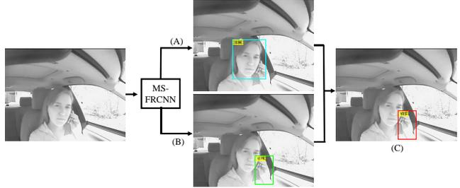
Figure 6. A flowchart of our cell-phone usage detection by applying the proposed MS-FRCNN (A): Face detection, (B) Hand detection, (C): cell-phone usage detection
