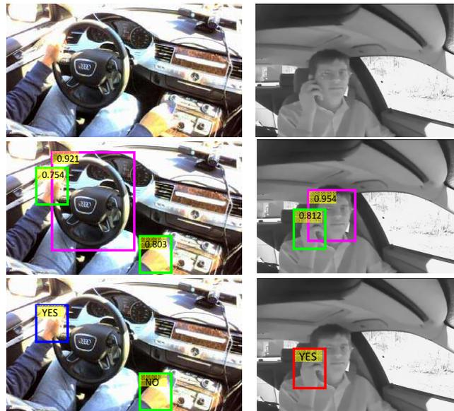
Figure 1. Our proposed Multiple Scale Faster-RCNN (MS-FRCNN) approach incorporating face detection and steering wheel detection problems into hand detection to determine whether driver's hands are on a steering wheel or not (the 1<sup>st</sup> column) or if a cell-phone is being used (the 2<sup>nd</sup> column).
