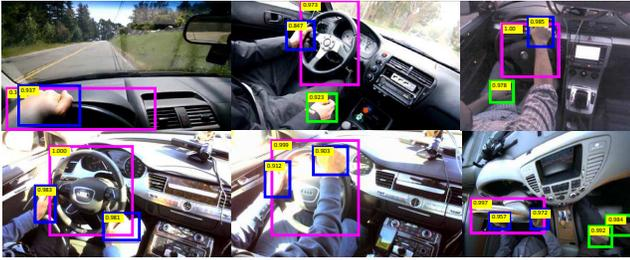
Figure 5. Some examples of our proposed hand on wheel detection method. The 1<sup>st</sup> row: one hand is on the wheel. The 2<sup>nd</sup>: both hands are on the wheel
