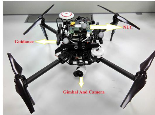
Figure 1. Our on-board platform: DJI Matrice 100 with Intel NUC (i5-4520u), DJI Guidance, DJI Zenmuse X3 gimbal and monocular camera.
