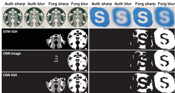
Figure 10. SVM and CNN results on SpLogo dataset. Both SVM classification and CNNs applied to the patches give false negatives on forged sharp edges, which are reduced significantly by applying the CNN to our histogram feature.
