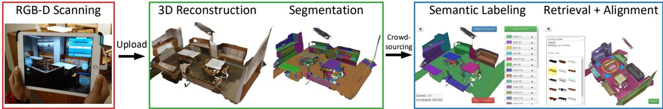
Figure 2. Overview of our RGB-D reconstruction and semantic annotation framework. **Left:** a novice user uses a handheld RGB-D device with our scanning interface to scan an environment. **Mid:** RGB-D sequences are uploaded to a processing server which produces 3D surface mesh reconstructions and their surface segmentations. **Right:** Semantic annotation tasks are issued for crowdsourcing to obtain instance-level object category annotations and 3D CAD model alignments to the reconstruction.
