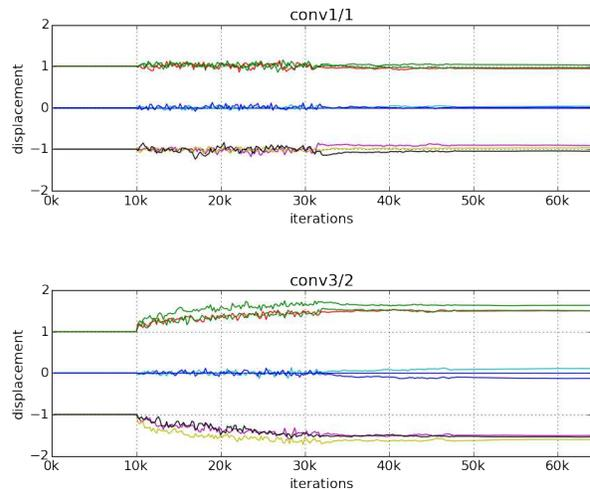
Figure 6. Movement of position. Each figure shows changes in the horizontal position ( $\alpha_k$ ) with iterations. Each figure shows the first and the last ACU layers. Each color represents one synapse (9 synapses in total).
