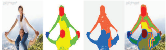
Figure 1. Our method finds human instances and the body part regions (arms, legs, torso, and head). From left to right: input image, semantic body part segmentation, person instance segmentation, final person individuation and part labeling.
