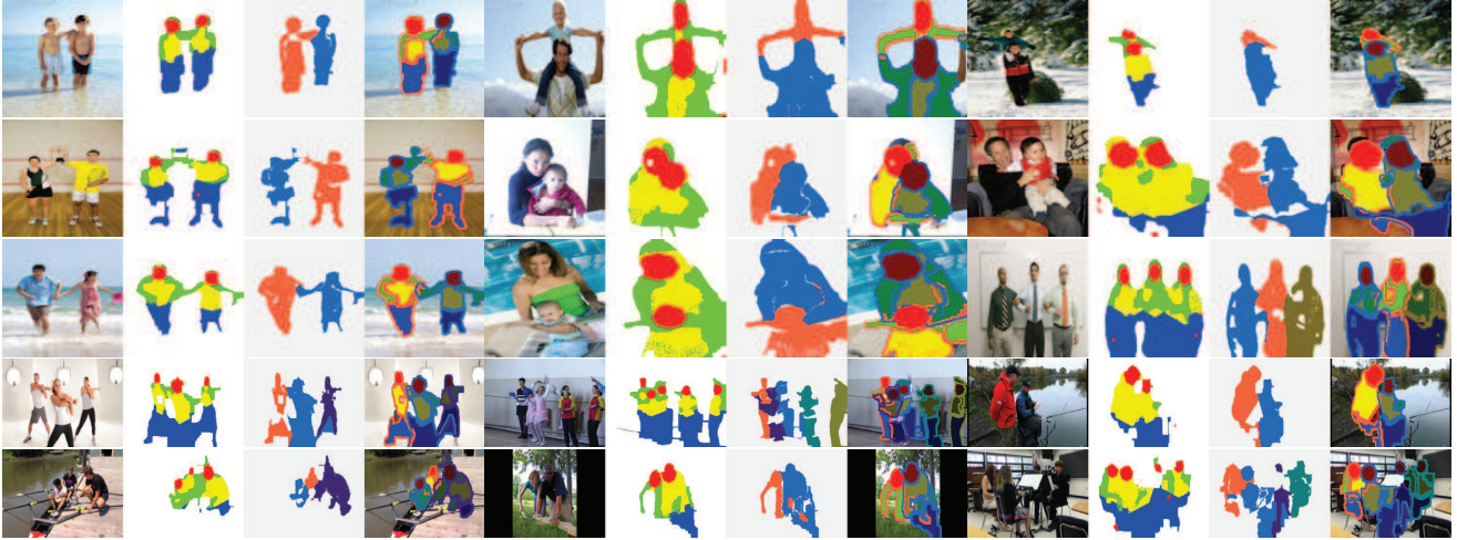
Figure 4. Sample results on the UCI and MPII datasets. Each result contains four columns: (1) the input images, (2) our input semantic segmentation body part map, (3) final instance segmentation, and (4) final body part segmentation using the proposed method. We use both shading and different boundary colors to show the segmentation. The same body parts have the same chromaticity (arm: green, leg: blue, torso: yellow, head: red) but have different brightness if they belong to a different person. All figures best viewed on pdf.
