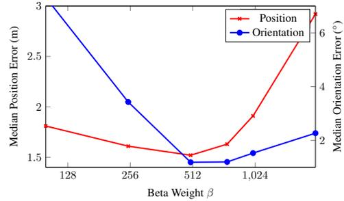
Figure 2: Relative performance of position and orientation regression on a **single model with a range of scale factors** for an indoor scene from the King’s College scene in Cambridge Landmarks, using the loss function in (2). This demonstrates that learning with the optimum scale factor leads to the network uncovering a more accurate pose function.
