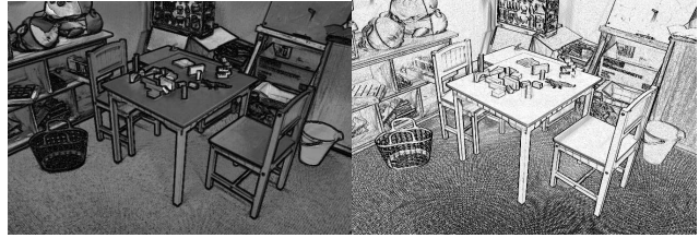
Figure 2: Learned vs fixed pairwise costs: Visualization of the pairwise costs between two neighboring pixels in horizontal direction using the learned Pairwise-CNN (left) and a fixed edge-function (right). Dark pixels indicate a low cost for changing the label and bright pixels indicate a high cost for a label-switch. Note, how the dark pixels follow object outlines (where depth discontinuities are likely) and how texture-edges tend to be suppressed ( e.g. , on the floor) in the learned version.
