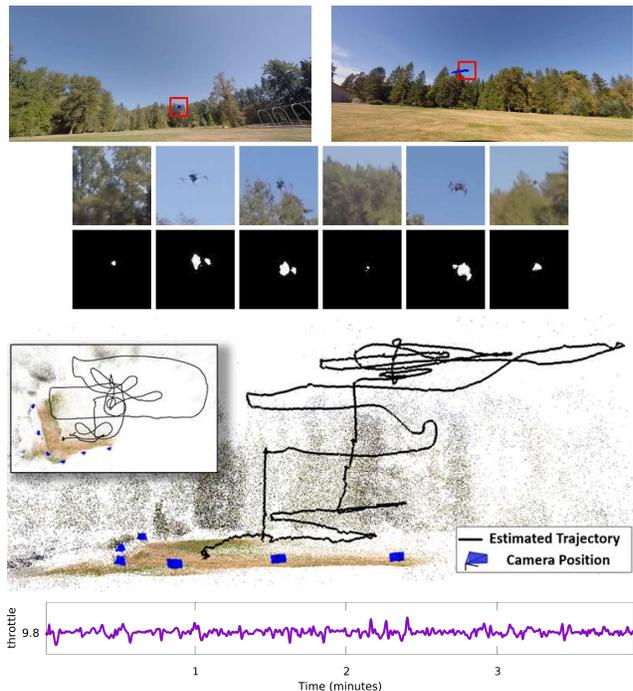
Figure 1: A quadrotor UAV was manually flown to a height of 45 meters above a farm within a  $100 \times 50m^2$  area with six cameras on the ground. [TOP] Two input frames along with the detections and zoomed-in views of the UAV are shown. [MIDDLE] 3D trajectory for a 4 minute flight and camera locations estimated by our method. The inset figure shows the top-down view. [BOTTOM] Estimated throttle signal (one of the control inputs sent to the autopilot).
