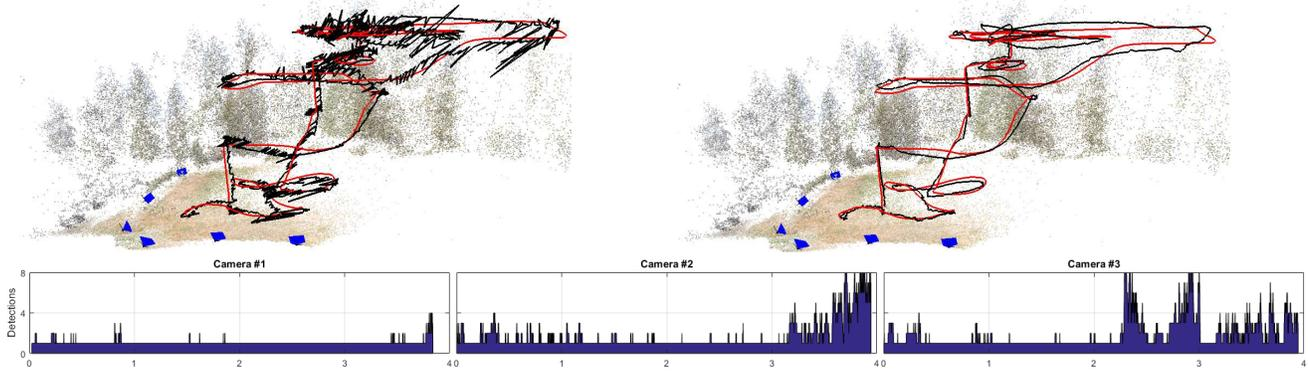
Figure 7: Qualitative Results (FARM dataset): The **black** and **red** curves denote the estimated and ground truth (GPS) trajectory respectively. [LEFT] Initialization trajectory estimate after the triangulation step. [RIGHT] The result obtained after bundle adjustment (BA-pDM). The trajectory is smoother and more accurate compared to the initial trajectory. [BOTTOM] The number of per-frame candidate detections for 3 videos. The middle and right plots show where tracking was difficult.
