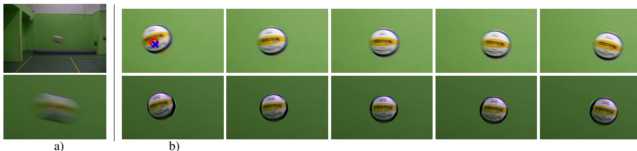
Figure 9: Reconstruction of an FMO blurred by motion and rotation. a) Input video frame. b) Top row: actual frames from a high-speed camera (250fps). Bottom row: frames at corresponding times reconstructed from a single frame of a regular camera (25fps), i.e. 10x temporal super-resolution. The top left image shows the rotation axis position estimated from the blurred frame (blue cross) and from the highspeed video (red circle).
