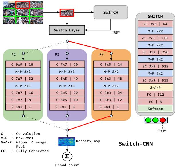
Figure 2. Architecture of the proposed model, **Switch-CNN** is shown. A patch from the crowd scene is highlighted in red. This patch is relayed to one of the three CNN regressor networks based on the CNN label inferred from **Switch**. The highlighted patch is relayed to regressor  $R_3$  which predicts the corresponding crowd density map. The element-wise sum over the entire density map gives the crowd count of the crowd scene patch.
