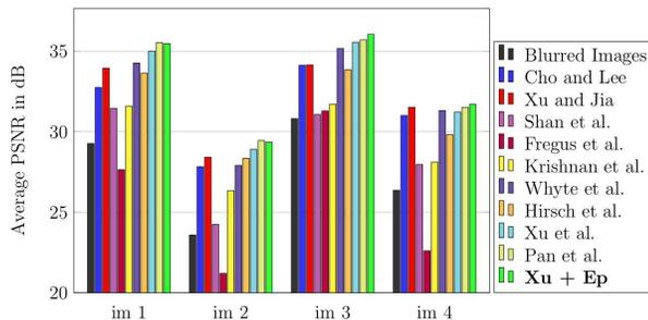
Figure 4. Quantitative evaluation on first 7 kernels from [13].
