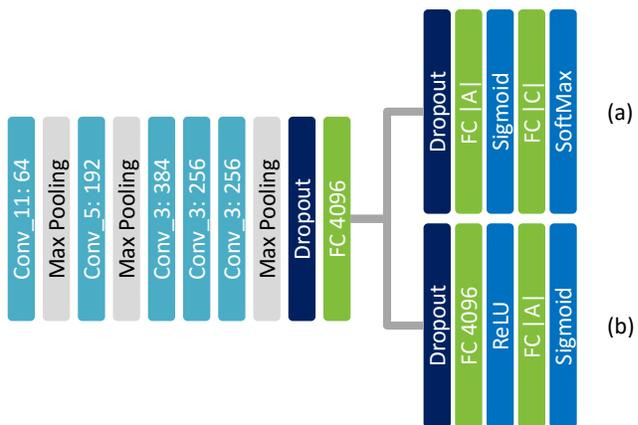
Figure 1: The detailed network architecture used for (a) the joint and (b) attribute models.
