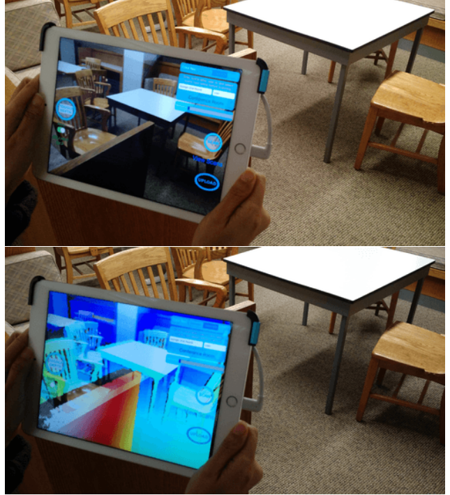
Figure 9. Our RGB-D recording app on an iPad Air2 with attached Structure sensor (showing color stream at the top and depth stream at the bottom). The app allows novice users to record RGB-D videos and upload to a server for reconstruction and annotation.
