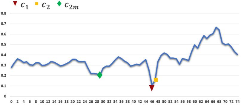
**Fig. 1.** Example of cost curve, showing the matching cost  $c_1$ , the second minimum  $c_2$  and the second local minimum  $c_{2m}$ . In this example, the disparity  $d_1$  is equal to 46.
