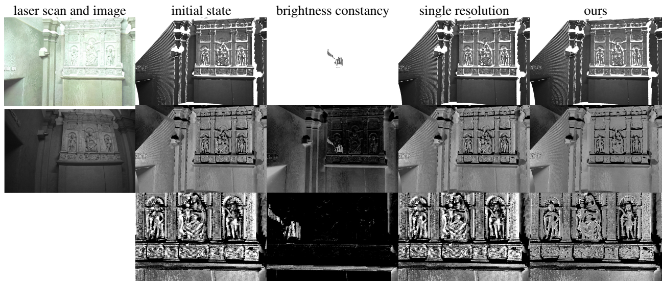
Figure 7: Comparison of different alignments for one image in the relief 2 scene. The laser scan is shown on the top left with its original colors, while the image to be aligned is shown below it. To the right of them, the laser scan is shown in the top row with the image projected onto it in different alignments. The middle row shows the difference image to the top left image, computed on grayscale images. In the bottom row, a cutout from the middle row is displayed with increased contrast. From left to right: Original laser scan colors and image, initial state (set manually for this example), alignment assuming brightness constancy, alignment with a single-resolution point cloud only, alignment using our complete method. Since the colors of the laser scan and the image differ strongly, a darker difference image does not necessarily mean that the alignment is better. Instead, the difference image being homogeneous is an indication for a good alignment. Note that when assuming brightness constancy, the camera intrinsics drift off such that only a small patch remains visible in the image.
