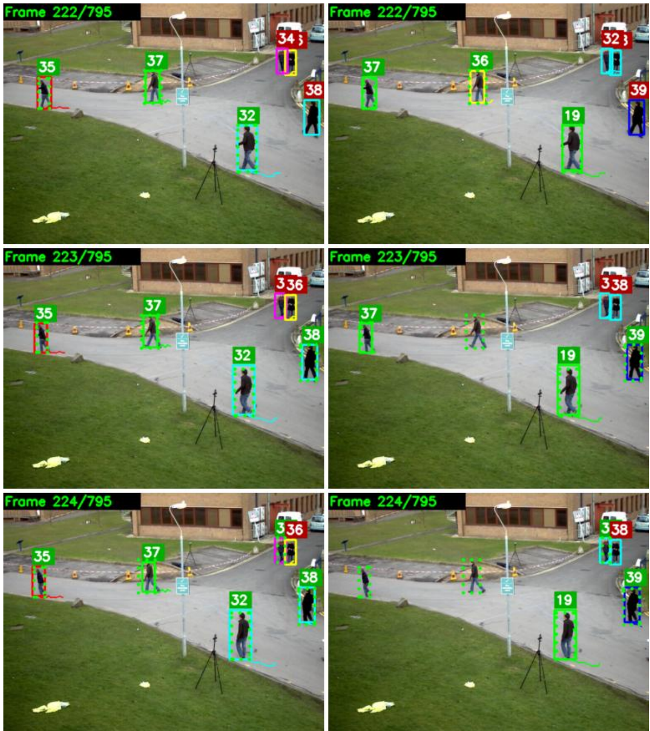
Figure 13: Left: model with only bounding box information as input for learning cost functions. Right: model with appearance features as input (raw RGB patches) for the unary term. In this failure case, the model using appearance features does not correctly track two pedestrians in the last two frames (object IDs 36 and 37).
