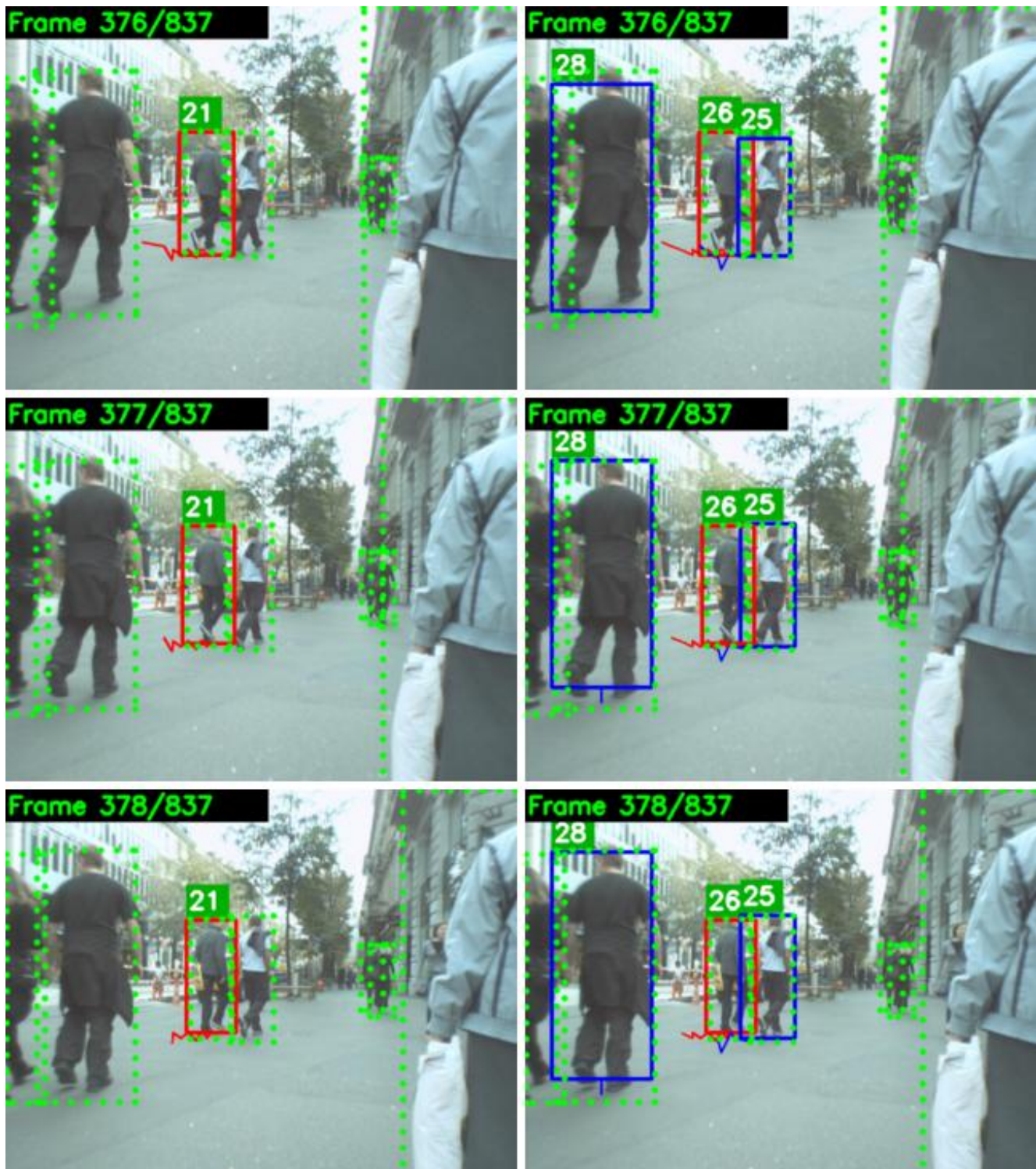
Figure 10: Left: model with only bounding box information as input for learning cost functions. Right: model with appearance features as input (raw RGB patches) for the unary term. The model using appearance features detects two more person (object IDs 28 and 25), while the other model misses them.
