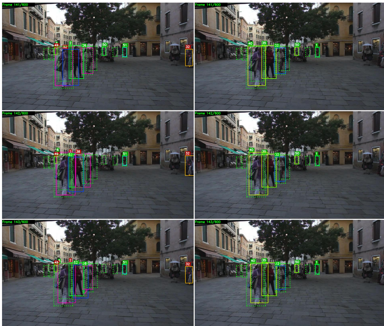
Figure 8: Left: model with only bounding box information as input for learning cost functions. Right: model with appearance features as input (raw RGB patches) for the unary term. Having access to appearance features seems to help in suppressing false positives from the underlying detector.
