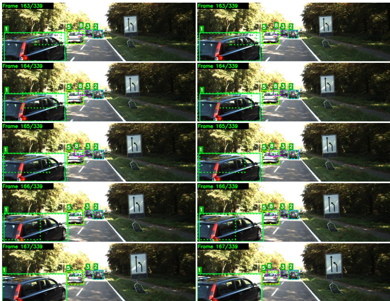
Figure 3: Left: model with hand-crafted costs. Right: model with learned costs from bounding box information. Note the failure case of the hand-crafted model in the last two frames in the middle part of the image. The car with the ID 8 is not tracked anymore.
