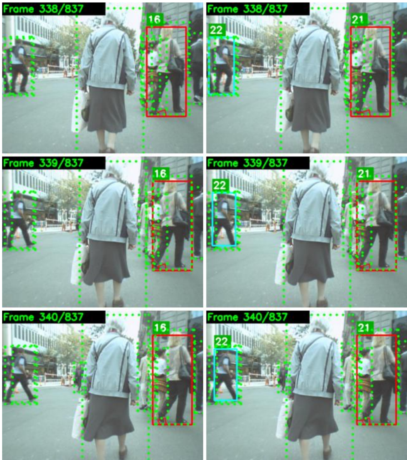
Figure 9: Left: model with only bounding box information as input for learning cost functions. Right: model with appearance features as input (raw RGB patches) for the unary term. The model using appearance features detects one more person on the left side of the image, while the other model misses it.
