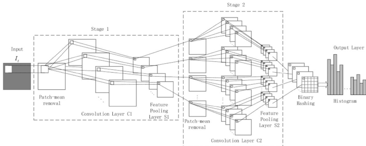
Figure 3: Basic structure of a three-stage PCN.
